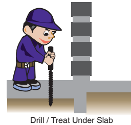
Drill / Treat Under Slab
